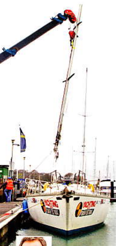
Hamble rigger Alan Moore unstepped the Crash Boat's masts at Hamble Point
